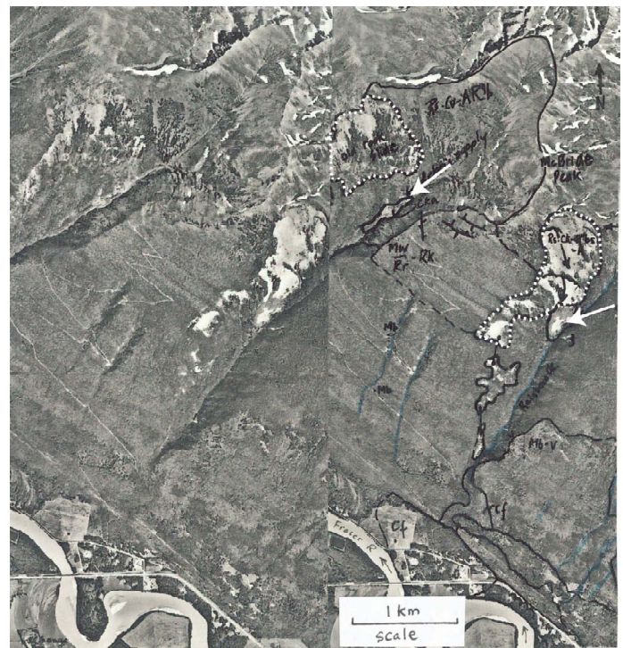
Figure 1 Stereogram of tributary watersheds along Robson Valley near McBride, B.C. Active rock fall (dotted) and abundant colluvium (arrow) in tributary valleys may contribute to debris flows or other hazards, which can travel downstream to impact facilities in the main valley.
