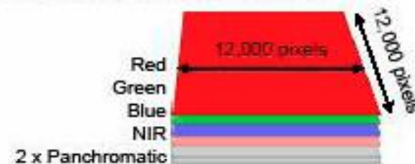
Single lens with a hypothetic surface array with six transparent layers for co-registration.
