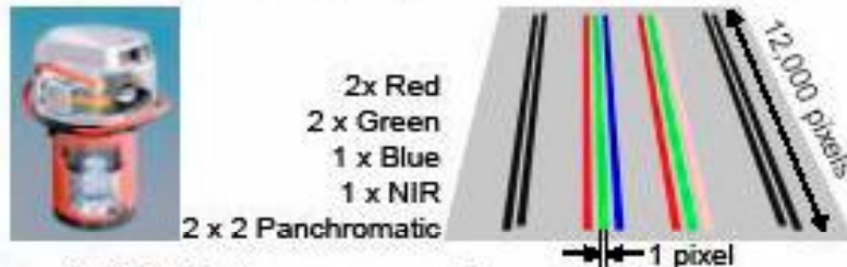
Single lens with a focal plate with 10 CCD lines. Trichroid features co-registration of spectral bands.
