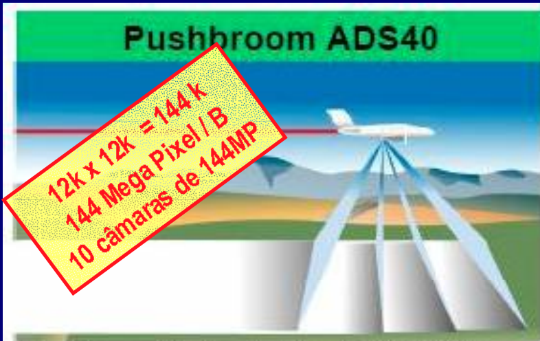
Single lens with a focal plate with 10 CCD lines. Trichroid features co-registration of spectral bands.
