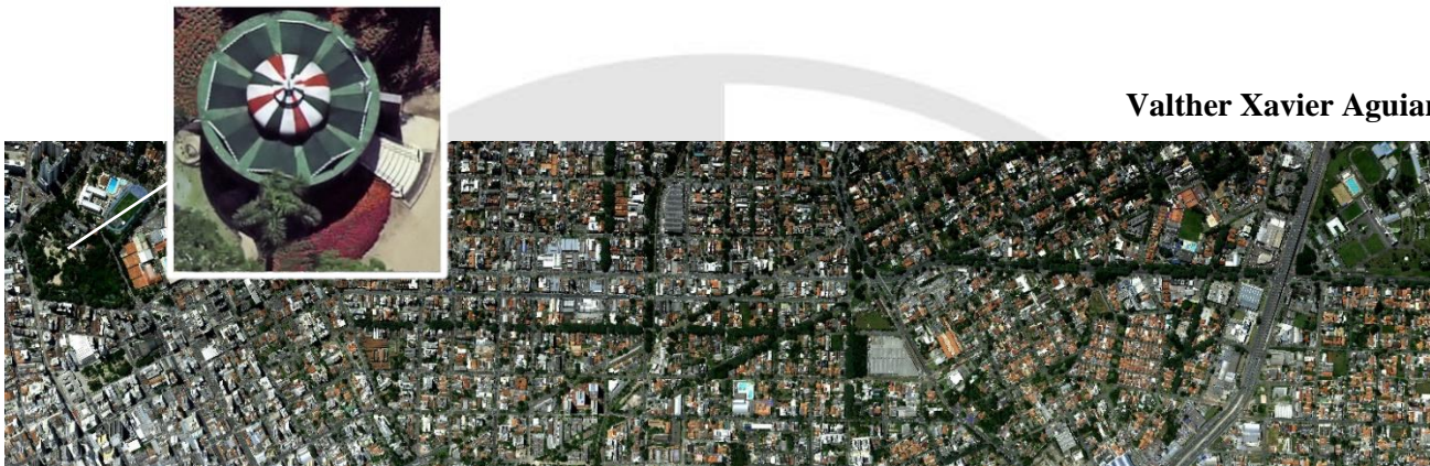
Zoom e parte do Carpet de Pixels obtido pelo sensor Leica ADS100 – GSD 5cm – 20.000 x 188.648 pixels – 3.773 megapixels – Curitiba
