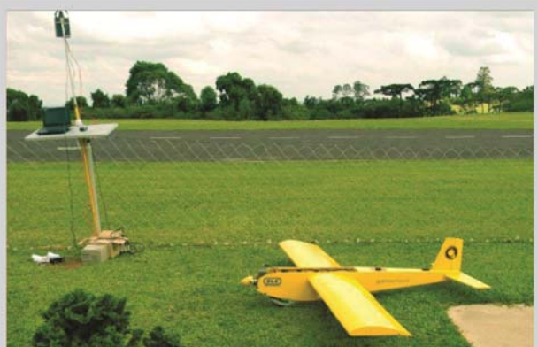
SIMEPAR / ESTEIO RPAS with 2-kg payload and small format sensor.
