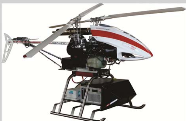
Swiss Drones RPAS with 35-kg payload and LEICA RCD30 medium format sensor.
