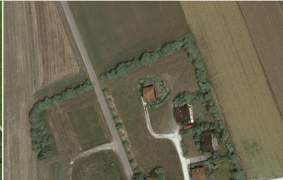
**Pan-sharpened based on spectral data with 22x lower area resolution**
