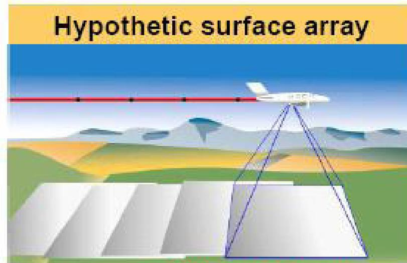
Single lens with a **hypothetical surface array** with six transparent layers for co-registration.
