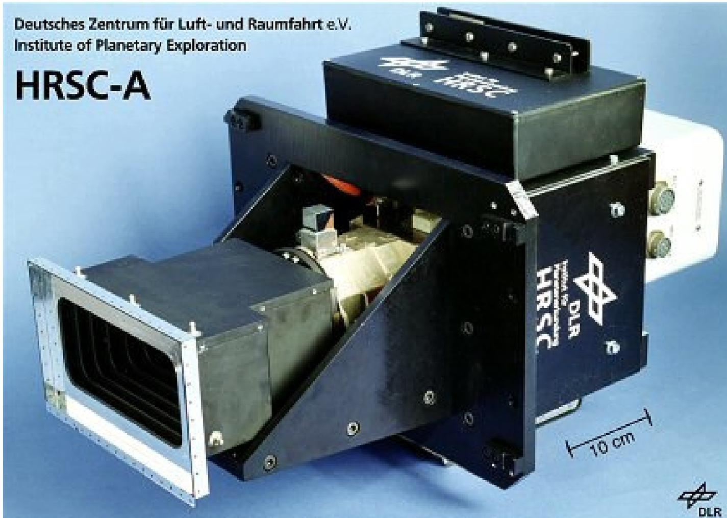
HRSC-A Line sensor Produced by DLR for the Mars96 mission later adapted for airborne applications for “proof of concept” testing.
