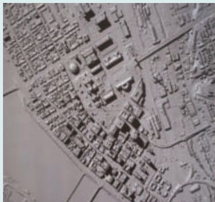
Figure 5. Digital Surface Model (DSM) derived from Leica ADS40 stereo imagery. Image courtesy of EarthData Inc.
