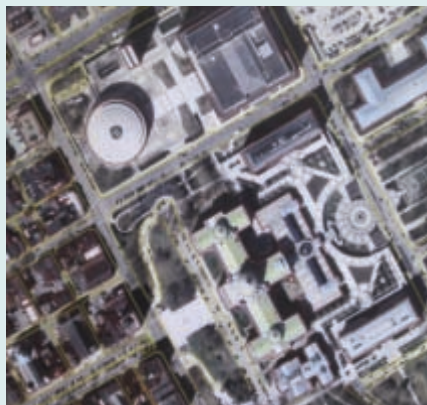
Figure 6. True orthophoto based on images and DSM derived from Leica ADS40 data. Image courtesy of EarthData Inc.
