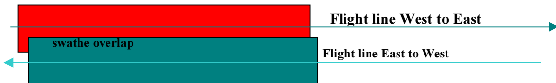
Figure 6 – Parallel swathes have an area of overlap (typically 25% of the swathe width)
