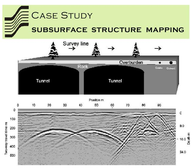
Ground penetrating radar locates the two tunnels shown in the diagram, represented by the two arches on the left side for the data set. The two shallower features on the right side are generated by a cable and culvert approximately one meter deep.
